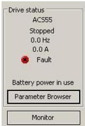
Figure 9. Drive status when the drive is battery-powered
