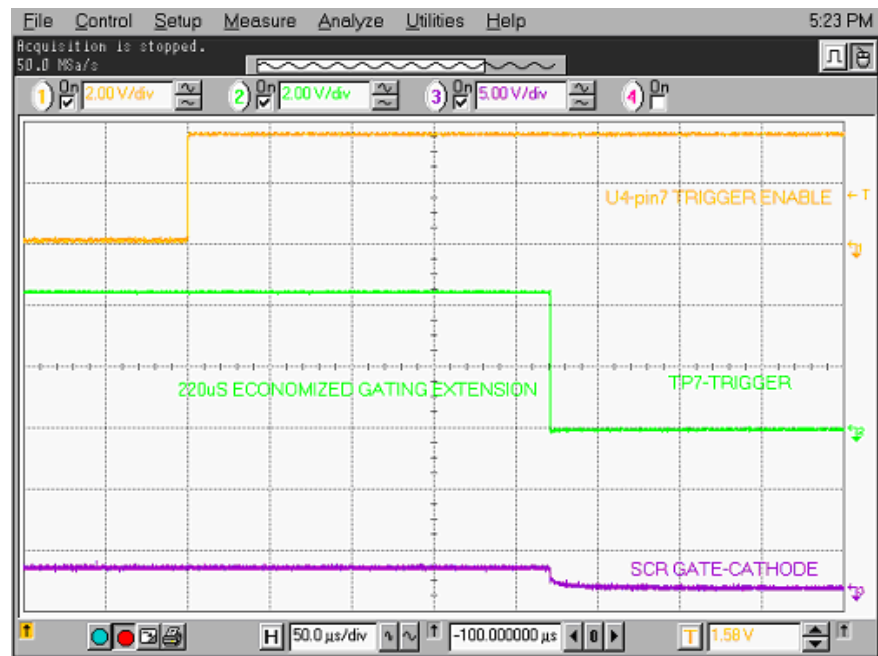
Figure 96 - Expansion of V Sense Trigger to SCR Gating Pulse
